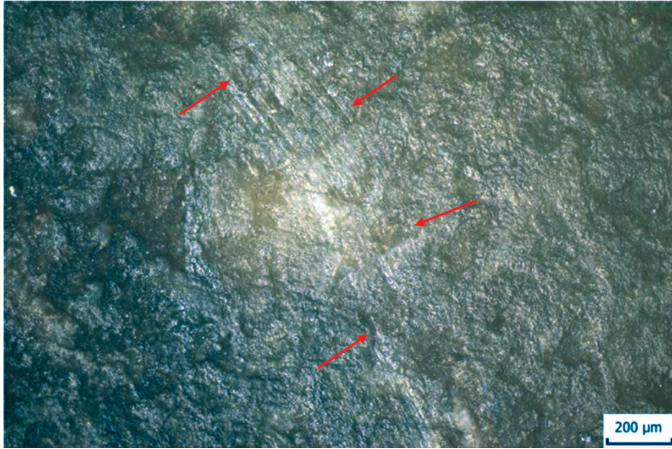
Fig. 4. Microtraces of Mitterberg-type binding on a stone grooved hammer from Dubicko (photo by author).
