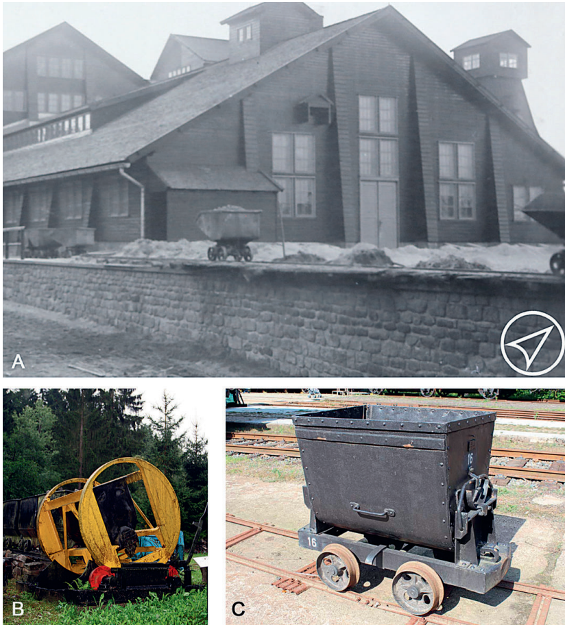
Fig. 9. A – Sauer sack/Rolava. Mining carts on the ramp south of the processing plant. The design of this type allows the hull to swivel and the load to be discharged to both sides ( StA Sachsen, BA Freiberg, Best. StB, Nr. 3-2847 ); B – analogy to swivel tipper (photo by A. Schwarz, source https://hellertal.startbilder.de ); C – mining cart, one of the types used according to written evidence at the Rolava mining plant (source https://www.vvm-museumsbahn.de/ix-start/ix-start.php?id=12&env=au&pname=/fz/C6/C64-Muldenk/C683-16/120916-IMG_2243-w1200m.jpg&pwidth=1200 ).
