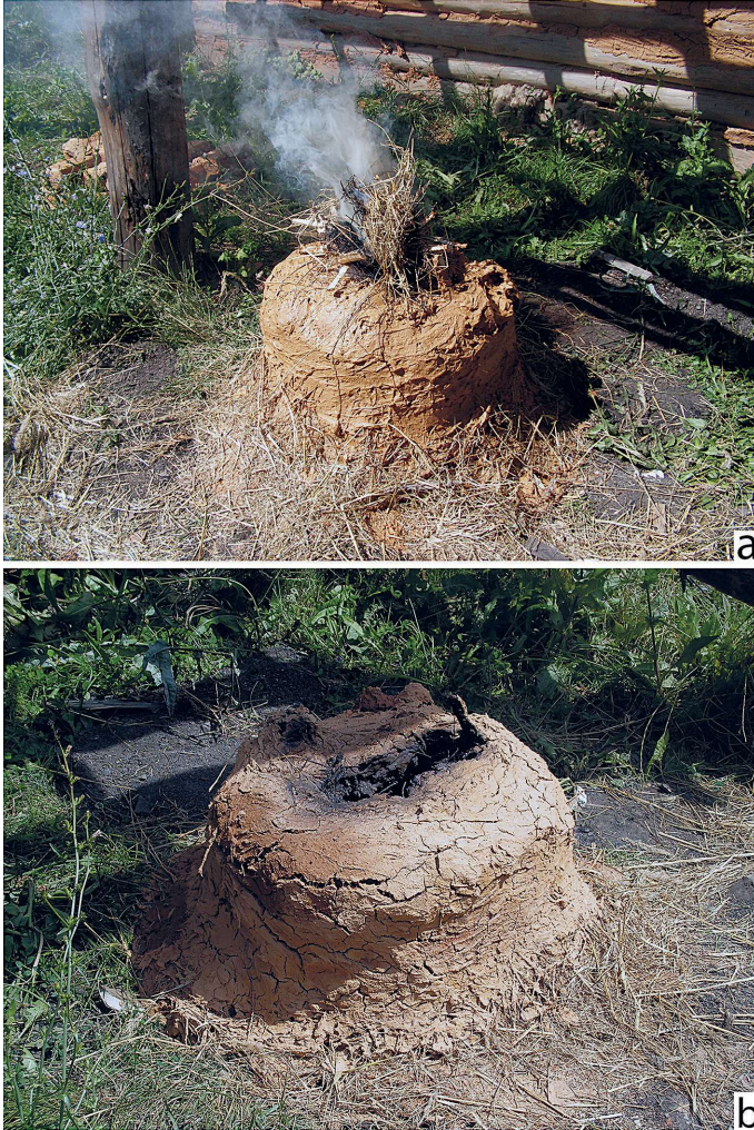
Fig. 6. Final stage of firing process in the pit kiln with a dome: a – sealing the dome with clay and potsherds; b – kiln at the end of firing (photo D. Łaciak).
