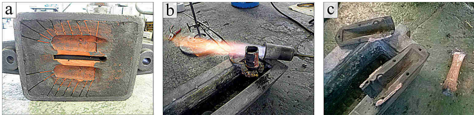
Fig. 11. The stages of the experimental casting of the Przedmieście type axe compatible with the casting mould from Elgiszewo: a – casting the mould; b – pre-heating the mould; c – knocking the casting out of the mould.
