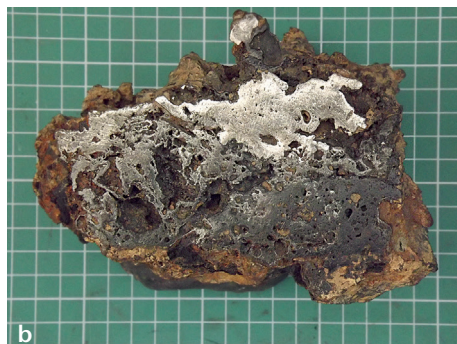
Fig. 3. Product of the experimental smelt I (Dymarki Świętokrzyskie 2013) in the form of bloom composed of 8 'segments' – view of the bottom side; below: schematic drawing of the bloom in the cross-section of the furnace shaft (a) and cross-section of one of the 'segments' (cells of the measuring grid have dimensions of 1 x 1 cm; b). Photo Kamila Brodowska (a) and Dariusz Kik (b).
