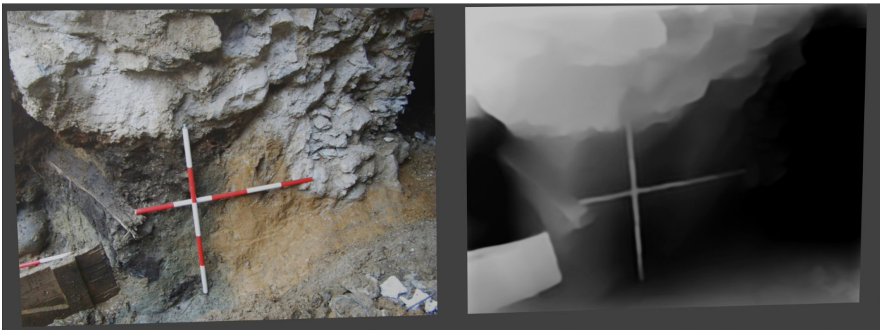
Fig. 2 Example of a depth map model
