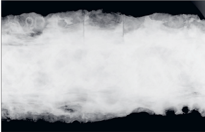
Fig. 14. X-ray image showing cracks in the cutting edge in the section where the blade is bent (by J. Hošek).
