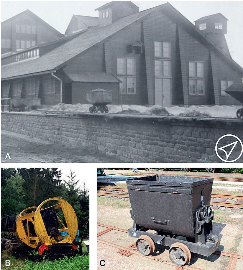
Fig. 9. A – Sautersack/Rolava. Mining carts on the ramp south of the processing plant. The design of this type allows the hull to swivel and the load to be discharged to both sides ( StA Sachsen, BA Freiberg, Best. StB, Nr. 3-2847 ); B – analogy to swivel tipper (photo by A. Schwarz, source https://hellertal.startbilder.de ); C – mining cart, one of the types used according to written evidence at the Rolava mining plant (source https://www.vvm-museumsbahn.de/ix-start/ix-start.php?id=12&env=au&pname=/fz/C6/C64-Muldenk/C683-16/120916-IMG_2243-w1200m.jpg&pwidth=1200 ).
