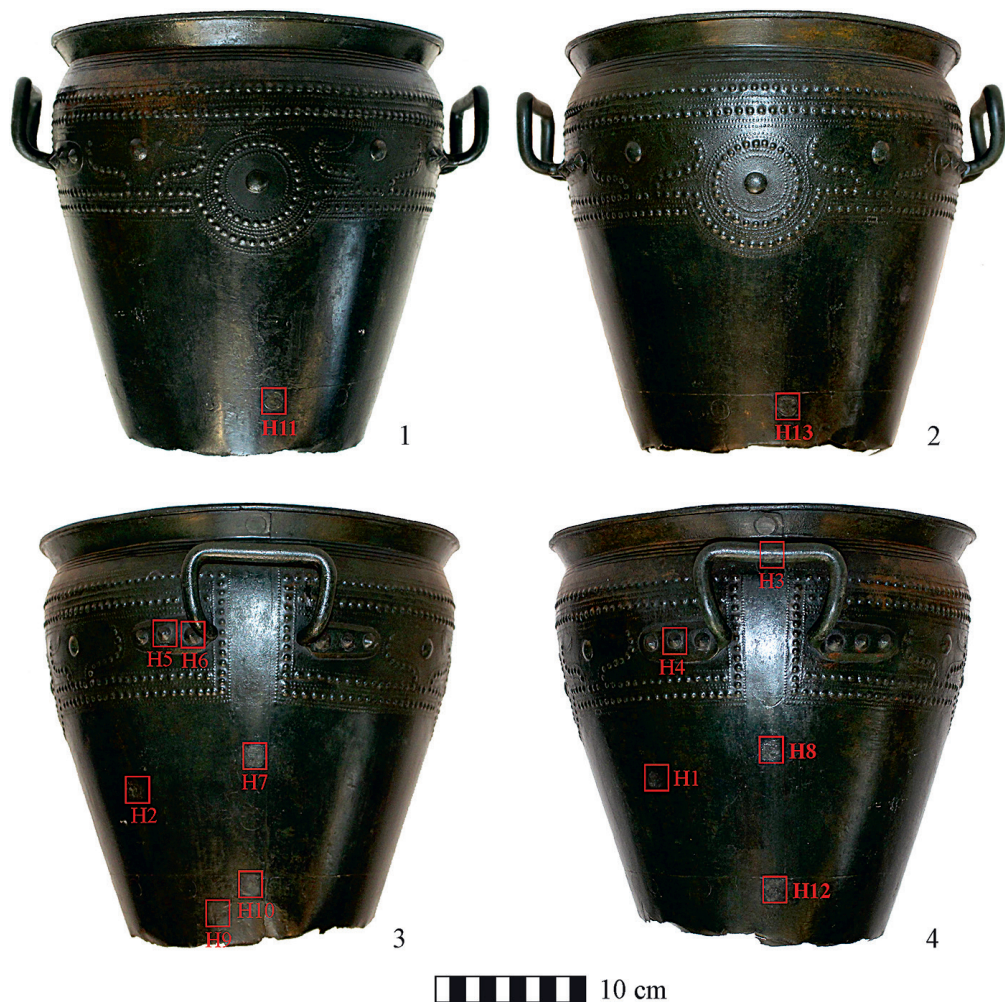
Fig. 3. Measured spots on the situla from Hajdúböszörmény-Csege-halom I hoard (Hungarian National Museum).
