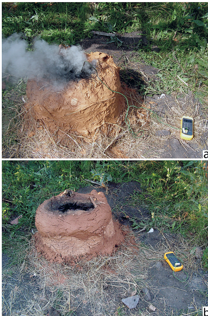
Fig. 7. Measurement of temperature in pit kiln with dome: a – at the beginning of firing and directly in the flame; b – at the end of firing (photo D. Łaciak).
